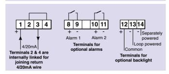
Output Isolated solid state switch complying with requirements for simple apparatus.  $5\Omega + 0.7V \text{ max}$ Ron Roff  $1M\Omega$  min
